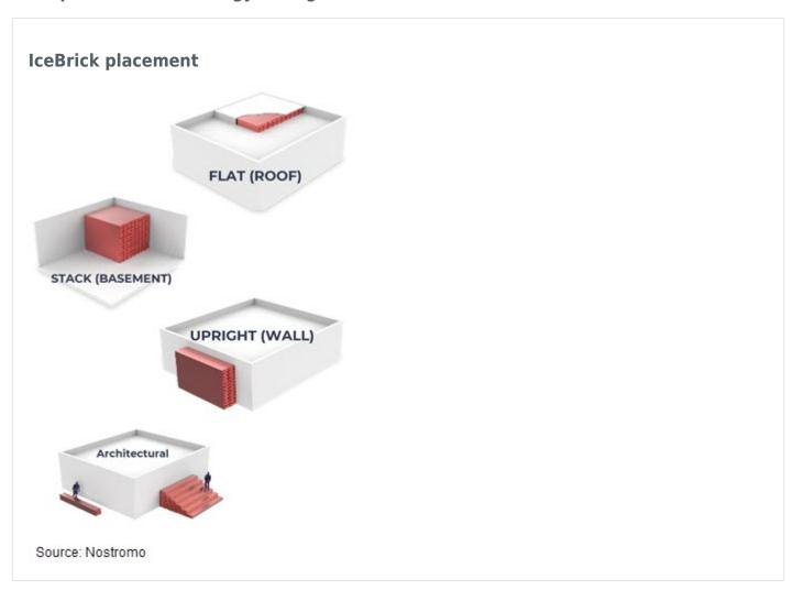
Nostromo's <u>IceBrick Energy Storage Array</u> is one example of innovative thermal energy storage packaging. (Another is <u>Viking Cold Solutions</u>.) Each brick holds the equivalent of 0.7–1.1 kW of energy. The IceBrick can be stored or stacked anywhere. It can even be incorporated into the building's architecture. The brick won't catch fire or leak harmful materials.
