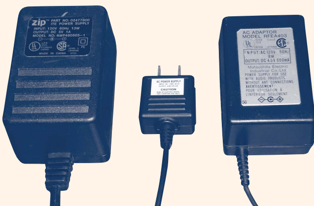
Figure 1: Smaller is better Efficient power supplies, such as the one in the middle, are lighter and more compact than typical power supplies on the market.
